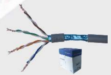
◎ XYD011 CAT-5 LAN CABLE STRUCTURE: PE INSULATION, FR PVC/LSOH PVC JACKET CONDUCTOR: FTP 4PAIRS SPECIFICATION: 24AWG REEL: 305M
