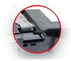
Gently remove the top of the device as shown.
