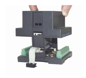
The jumpers are shown at right. Change the jumper settings as required, in accordance with the tables shown on the next page.
