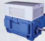
Compressor Drive Motor - up to 2000HP - 2pole, ODP, WP I & II - 2300~14000V, 60Hz
