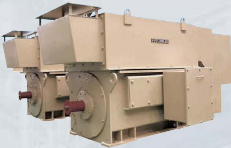
HV Induction Motor (HRQ7 Type) - Totally-enclosed Air to Air Cooled Machine - 1300~10000HP/4pole, 6.6kV, 60Hz
