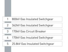
The SF<sub>6</sub> Gas Insulated Switchgear(GIS) contains the major equipment used in a substation such as a gas circuit breaker, disconnecting switch, earthing switch, voltage transformer, current transformer, lightning arrester, etc. in a grounded, metallic enclosure. The switchgear is filled with SF<sub>6</sub> gas, which has the best insulation and arc-quenching capabilites.
