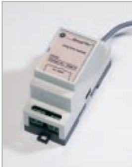
This external DIN-rail mounted device with modular dimensions is directly connected to the SMR1 electronic trip unit. The device is equipped with a NC 1A/400V AC contact that opens to a signal which indicates that a LT trip will shortly be initiated by the SMR1. The SMR1 emits this
