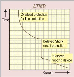
This trip unit offers overload and short-circuit protection. The overload protection is adjustable from 0.8 to 1 x the chosen rating whilst the short-circuit protection is set at 10 x the chosen rating (FD frame) or adjustable from 5 to
