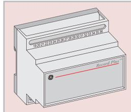
This external DIN-rail mounted device with modular dimensions is directly connected to the SMR2 electronic trip unit. The device is equipped with four NC 1A/400V AC contacts that can be
