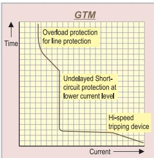
A trip unit designed to offer overload and short-circuit protection. The overload protection is adjustable from 0.8 to 1 x the chosen rating whilst the short-circuit protection is set at about 4 x the chosen rating (FD frame) or
